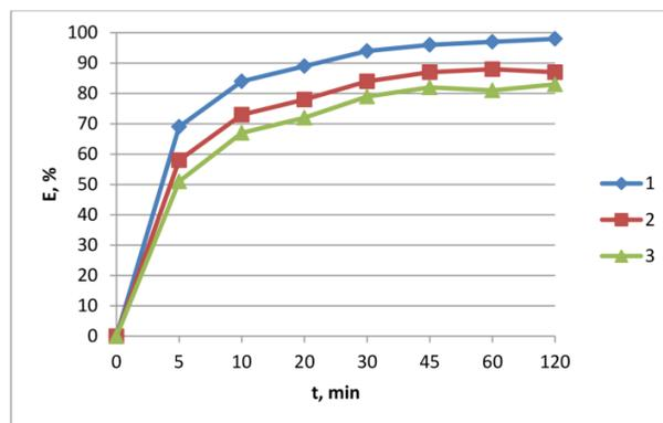
**Fig. 7.** Efficiency of sedimentation from the time of treatment of biodegradable organic waste with various reagents: 1-oxalic acid, 2-phosphogypsum, 3 - superphosphate.
