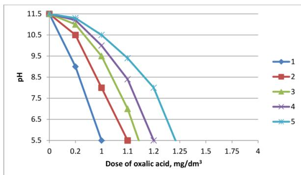
**Fig. 6.** The dependence of pH on the dose of oxalic acid with different dry matter content in biodegradable organic waste 1-2%, 2-4%, 3-6%, 4-8%, 5-10%
