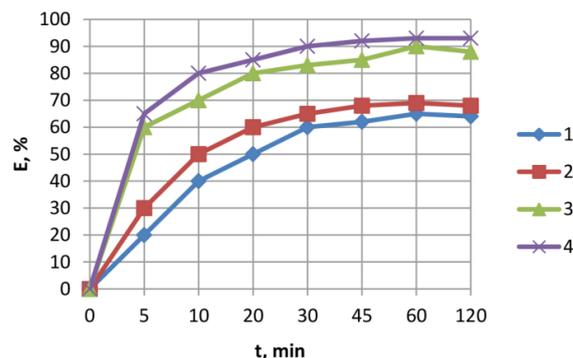
**Fig. 2a.** The effectiveness of sedimentation of biodegradable organic waste from processing time at doses of slurry suspension CaC<sub>2</sub>, g/dm<sup>3</sup>: 1-1, 2-1.5, 3-2.5, 4-3
