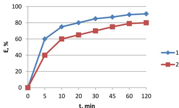
**Fig. 2b.** Efficiency of sedimentation of biodegradable organic waste from the time of treatment with a  $\text{CaC}_2$  suspension during sedimentation in cylinders with a diameter, mm: 1-0.65; 2-0.45
