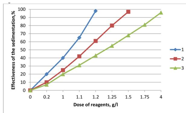
**Fig. 8.** Dependence of the effect of sedimentation on the dose of acidifying reagents 1 - oxalic acid, 2 - phosphogypsum, 3 - superphosphate
