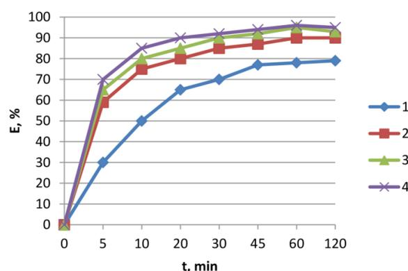
**Fig. 3.** The efficiency of the separation of biodegradable organic waste into liquid and solid fractions at a dose of oxalic acid  $1.0 \text{ g/dm}^3$  of temperature,  $\text{C}^\circ$ : 1-10, 2-20, 3-30, 4-40
