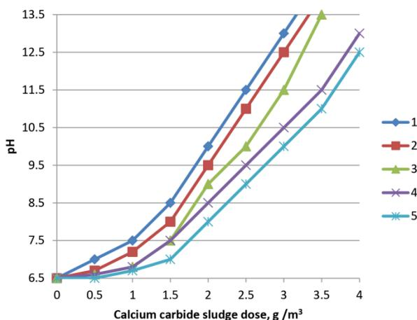
**Fig. 5b.** Change in pH of a dose of a suspension of  $\text{CaC}_2$  sludge and the percentage of dry matter in organic waste: 1-2.5%, 2-4.5%, 3-6.5%, 4-8.5%, 5-10.5%
