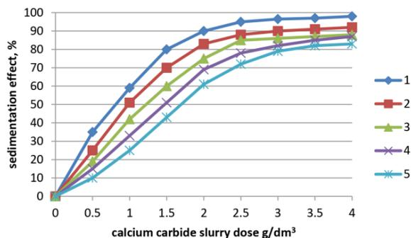
**Fig. 5a.** Efficiency of separation of biodegradable organic waste from dose with a slurry suspension of  $\text{CaC}_2$  and the percentage of dry matter: 1-2.5%, 2-4.5%, 3-6.5%, 4-8.5%, 5-10.5%
