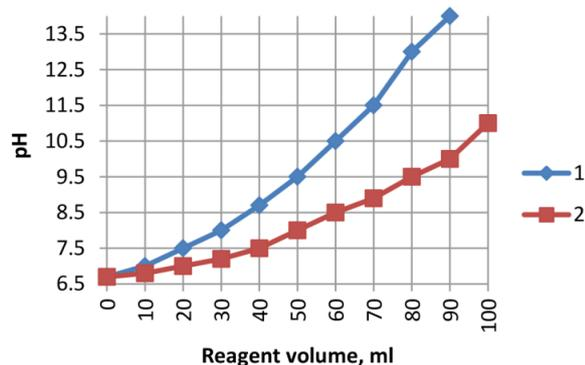
**Fig. 1.** The pH value of biodegradable organic waste (1dm<sup>3</sup>) after clarification of the volume of the reagent: 1-10% suspension of Ca(OH)<sub>2</sub>; 2 - 10% slurry suspension CaC<sub>2</sub>
