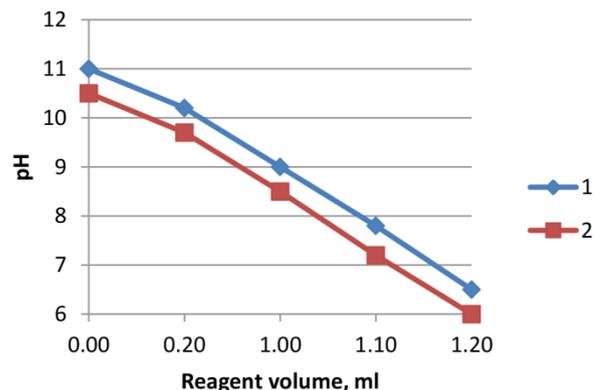
**Fig. 4.** Changing in pH of the mixture depending on the volume of oxalic acid solution at pH of biodegradable organic waste after treatment with 10% slurry suspension  $\text{CaC}_2$  ( $1 \text{ dm}^3$ ) 1-11.0 2-10.0
