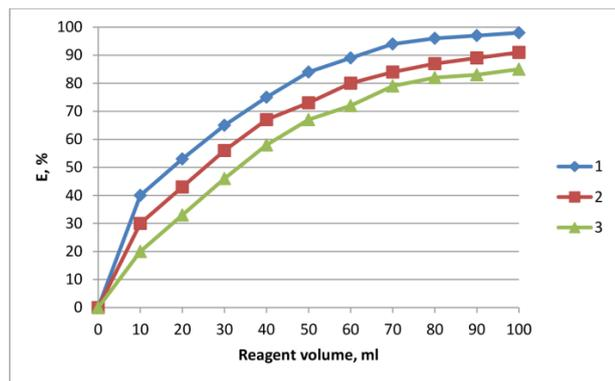
**Fig. 9.** Dependence of the effect of sedimentation on the volume of the reagent 1 - oxalic acid, 2 - phosphogypsum, 3 - superphosphate
