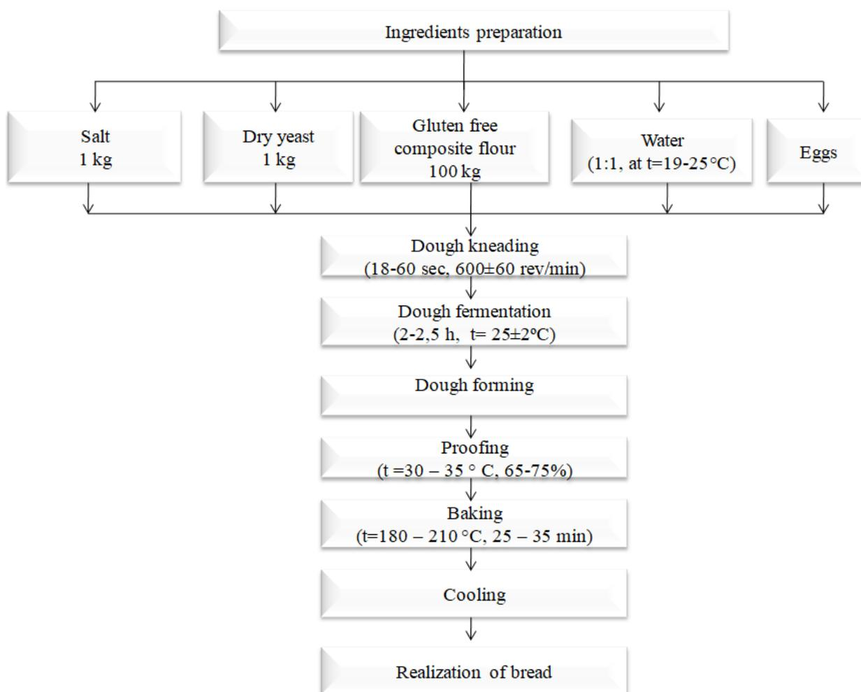
**Fig. 2.** Gluten free bread process flow diagram
