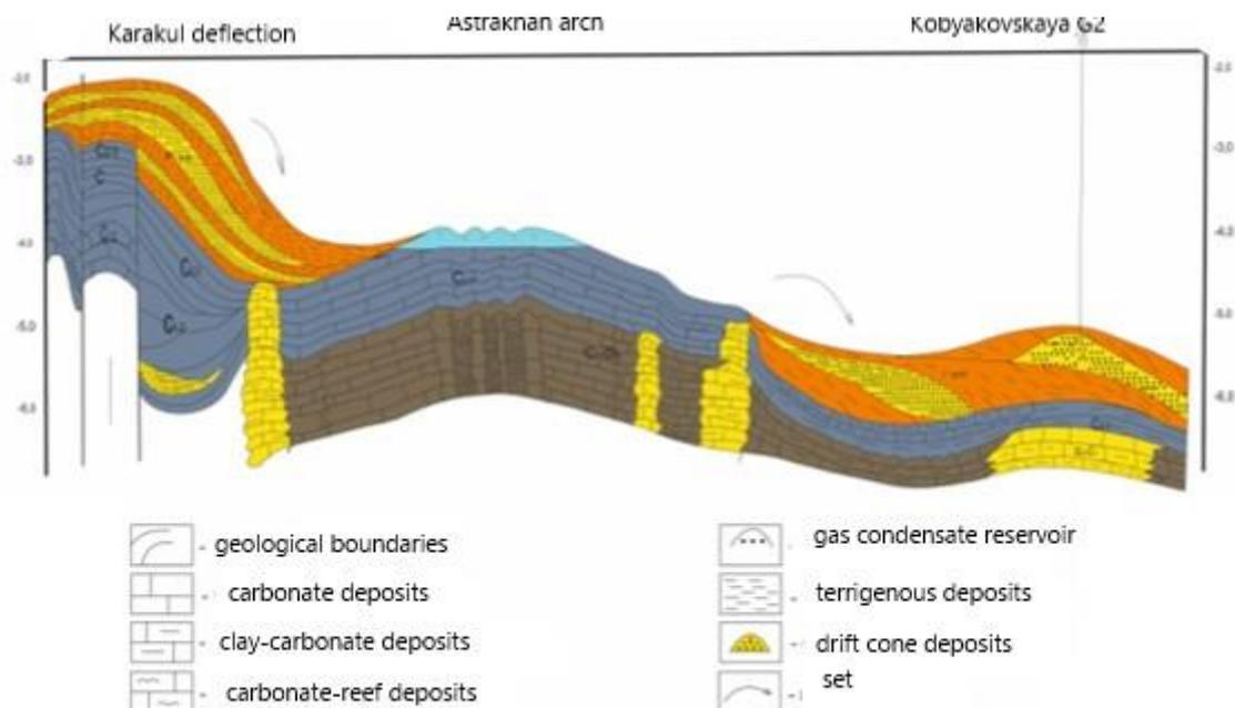
**Fig. 3.** Scheme of the formation of subsalt structures in the south of the Pre-Caspian basin along the Karakul trough - Kobyakovskoe uplift (according to the data of O.S. Obryadchikov, 1998; with additions of K.M. Taskinbaev, 2007)
