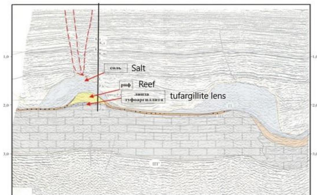
**Fig. 7.** Seismogeological section and trap model on the Kairan structure.
