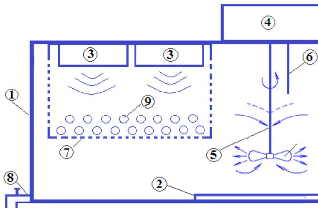
**Fig. 1.** Diagram of the proposed design of the plant raw material extractor
