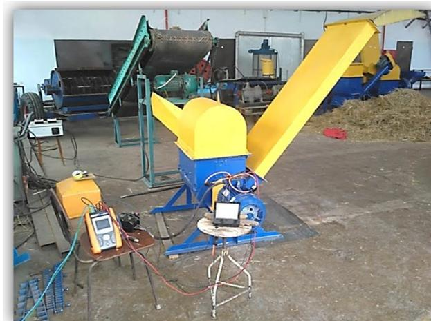
1 - belt conveyor; 2 - universal crusher DU-11; 3 - electric power quality analyzer AKE-824
