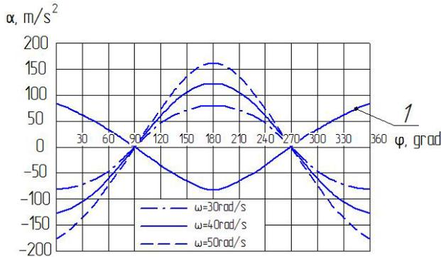
**Fig. 4.** Graph of the change in acceleration  $\alpha$  of the knife with double mileage and (1) the opposite end of the rocker depending on the angle and turning the crank  $\varphi$
