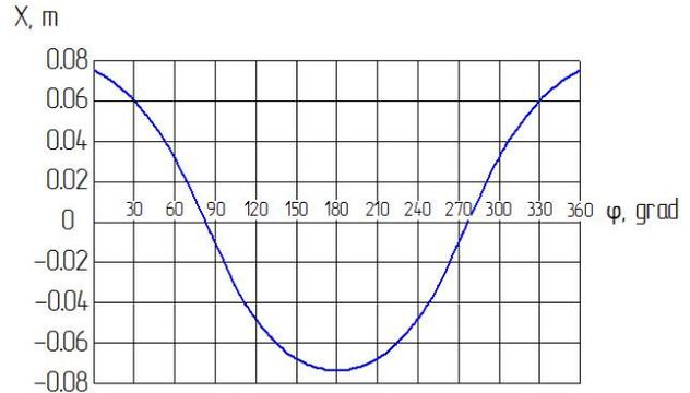
Fig. 2. Graph of the movement of the knife  $x$  with double mileage depending on the angle and rotation of the crank  $\varphi$
