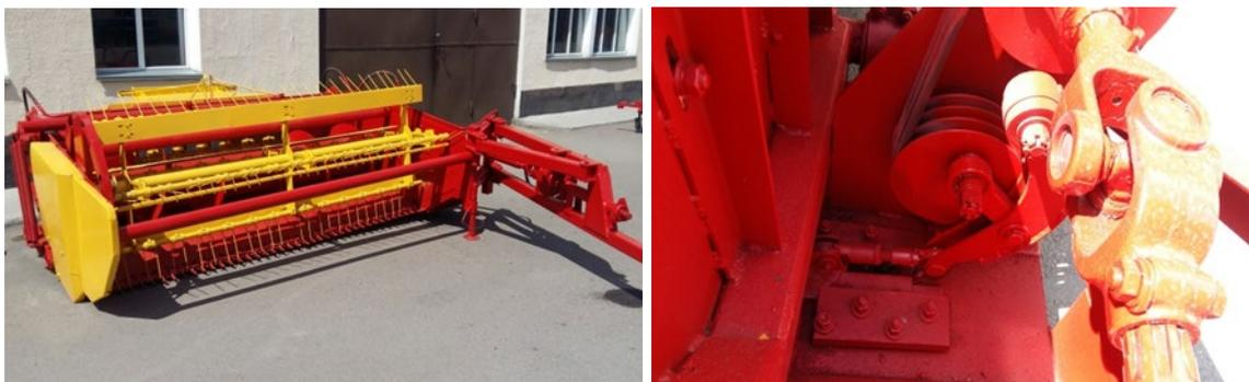
**Fig.5.** Crank-beam mechanism for the drive of cutting device with a double stroke, used in the KP-3,0 mower conditioner
