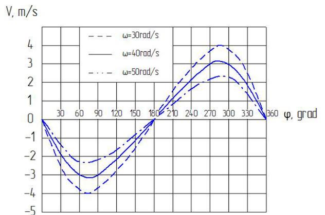
Fig. 3. Graph of the speed of the knife  $v$  with double mileage depending on the angle and rotation of the crank  $\varphi$
