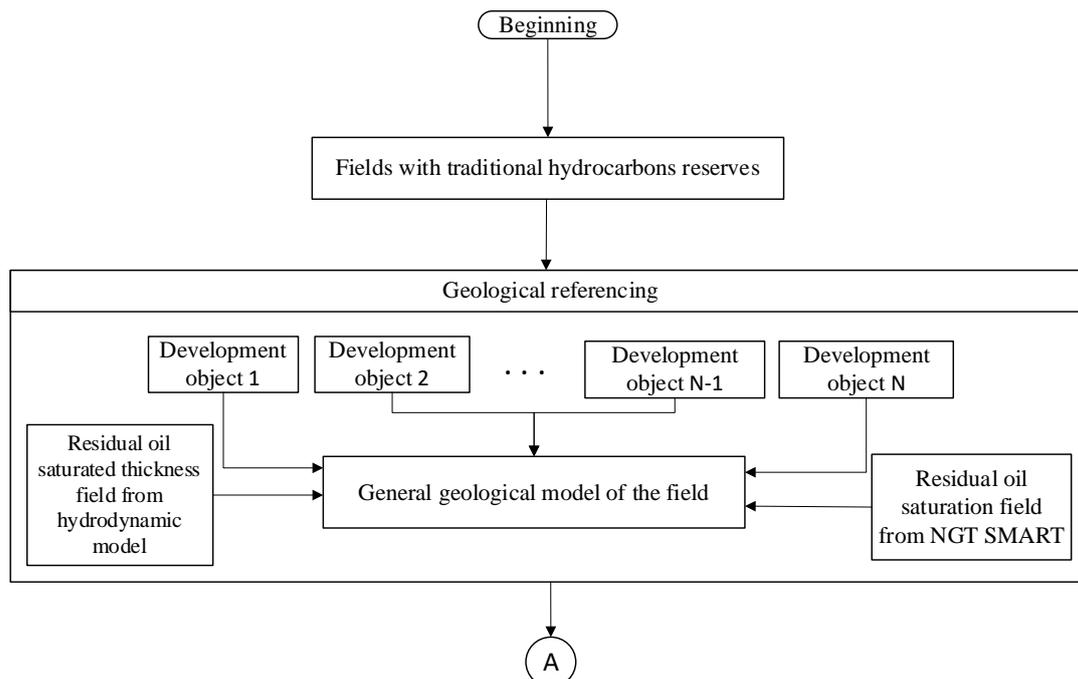
**Fig. 2.** Algorithm for the formation of many development scenarios for deposits
