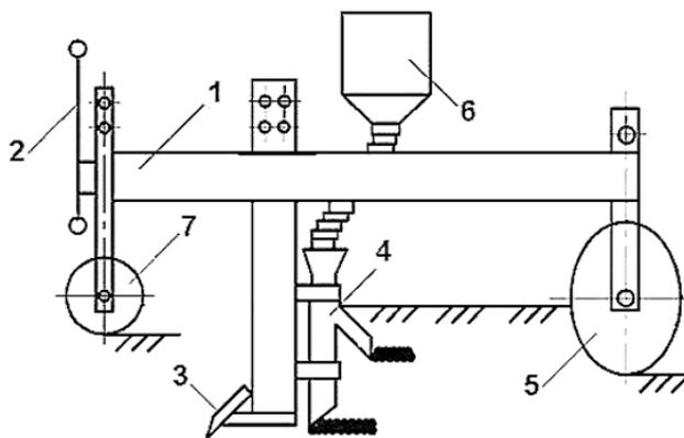
1 - frame; 2 - hitch; 3 - ripper tooth; 4 - Coulters for two-layer tape fertilizer application; 5 - spherical disk
