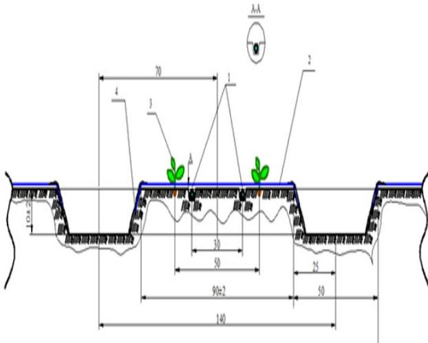
1 - drip irrigation tape; 2 - mulch film; 3 – seedling of vegetable crops; 4 - part of the mulch film embedded by the soil.
