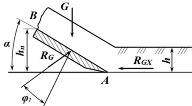
**Fig. 3.** Scheme for the determination of traction resistance arising from the lifting and moving the soil on the working surface of the ripper
