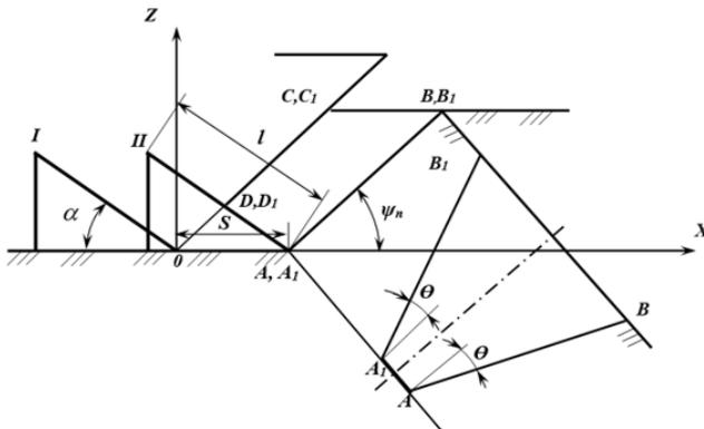
**Fig. 4.** The process of deformation and destruction of the soil under the influence of ripper
