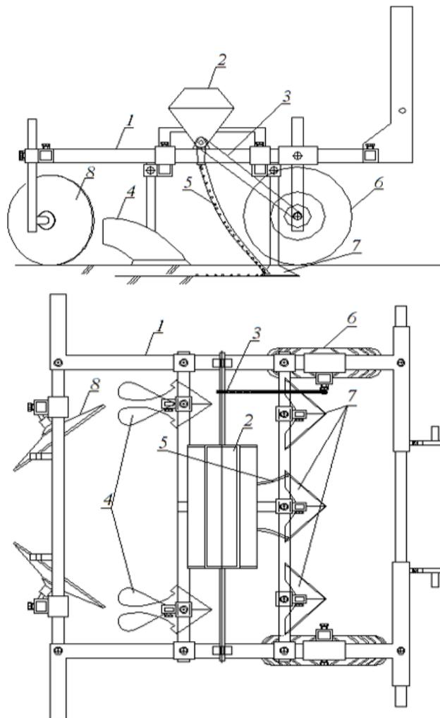
1-frame; 2- fertilizer hopper; 3 – mechanism of fertilizer gear; 4 - right-left harvester bodies; 5 - opener for double-layer tape fertilizer application; 6-wheel, 7-ripper; 8-spherical disks.
