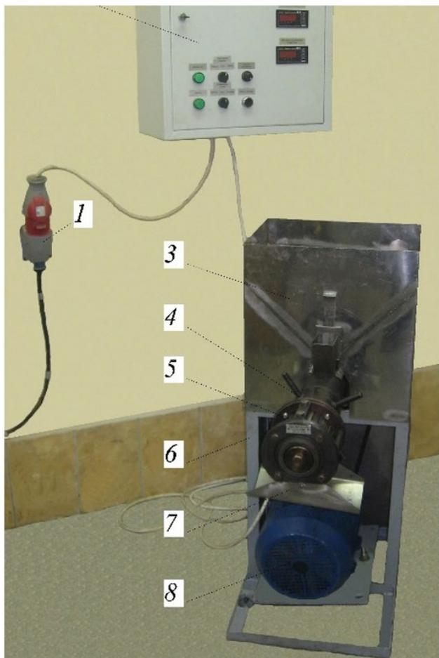
**Fig. 2.** Experimental installation of MPE-1: 1 - power supply; 2 - control panel, 3 - charging hopper; 4 - regulating device of the clearance; 5 - pressing chamber; 6 - mount; 7 - oil collector; 8 - electric coupling
