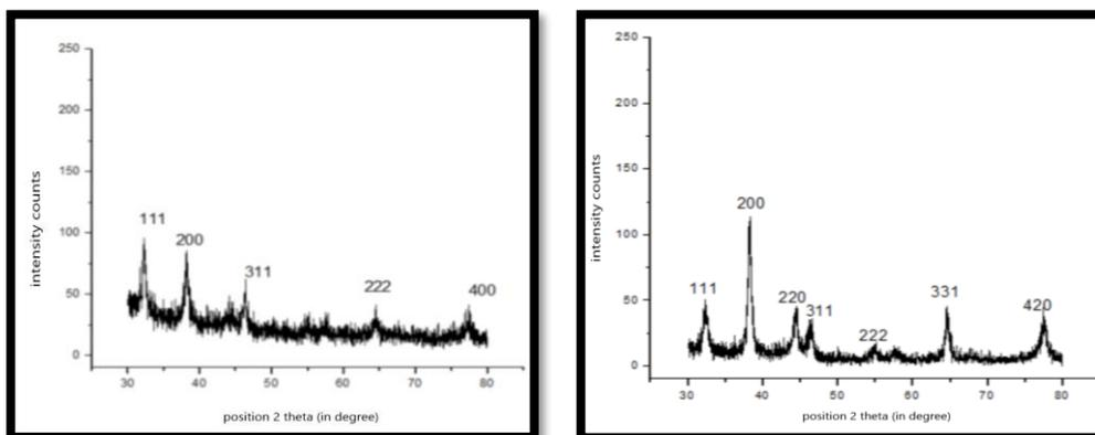
**Fig. 4.** XRD pattern of silver nanoparticles Which Synthesis From Hot and Ethanolic Extract
