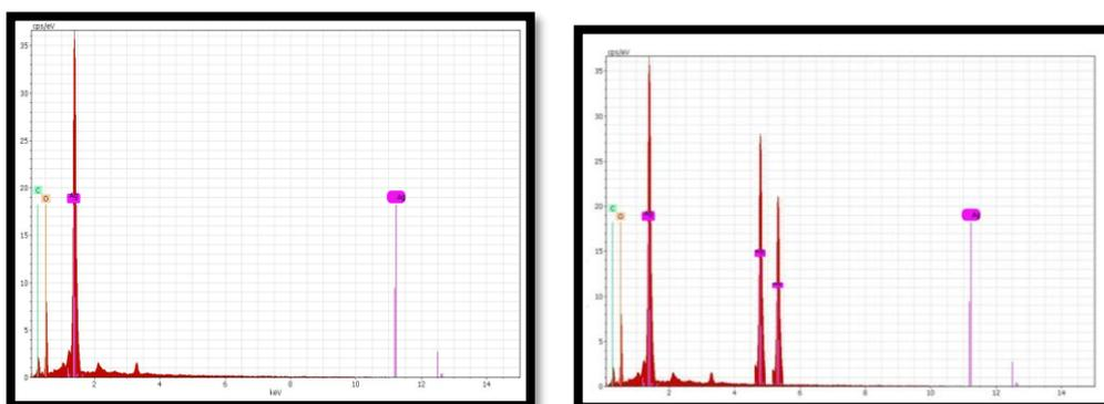
**Fig. 7.** EDAX spectrum of AgNPs Which Synthesis From Hot and Ethanolic Extract
