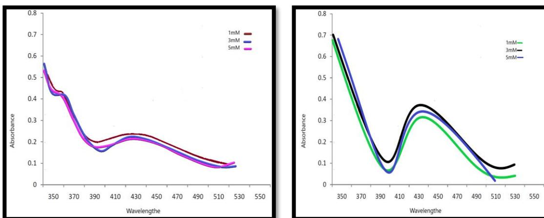
**Fig. 3.** UV Spectrum of Synthesis of silver Nanoparticles at different concentration of silver nitrate
