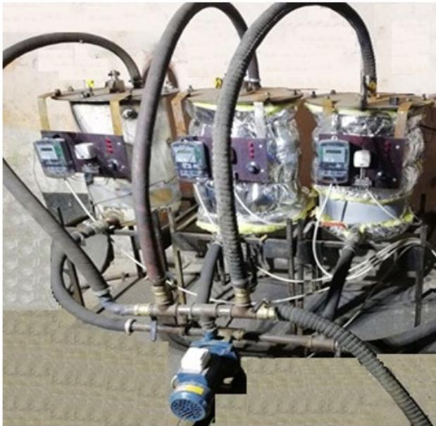
**Fig. 4.** Laboratory installation of a three-stage bioreactor
