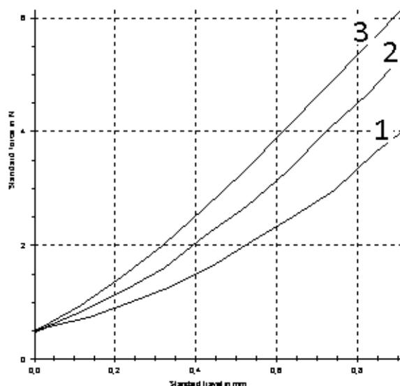
**Fig. 7.** “Force – Travel” diagrams for the different types of the studied models: 1 – model type B; 2 – model type C, 3 – model type D
