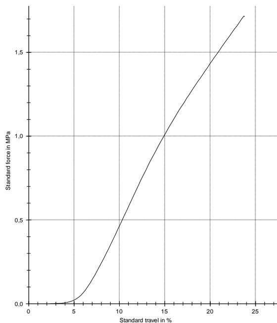
**Fig. 4.** Strain diagram of filled polydimethylsiloxane, which is generally used for modelling the nasal septum cartilage properties
