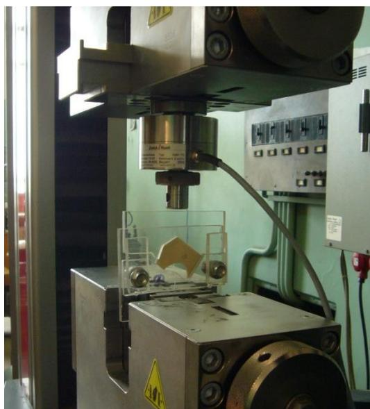
**Fig. 6.** Device for measuring the stiffness of nasal septum models in the grip of the ZWICK Z100 instrument
