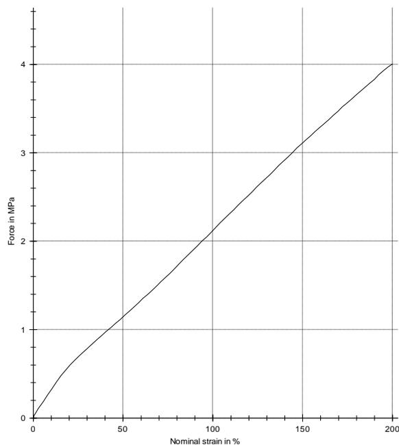
**Fig. 3.** Strain diagram of filled polydimethylsiloxane, which is generally used for simulating the nasal septum cartilage properties
