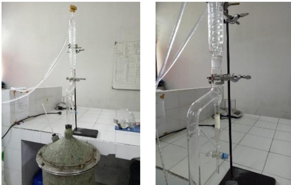
**Fig. 2.** Essential Oil Distillation Process from Nutmeg Fruit Flesh
