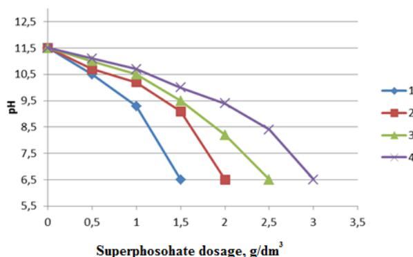
**Fig. 7.** Dependence of pH on ammophos dose at solid matter content: 1-1%; 2-3%; 3-5%; 4-7%
