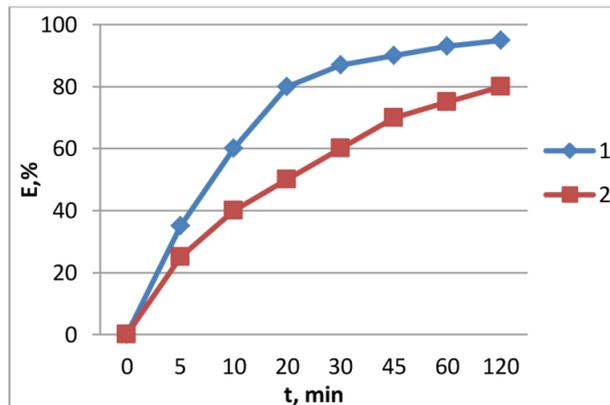
**Fig. 3.** Dependence of the retention effect on time at different cylinder diameters, mm: 1- 100; 2-45
